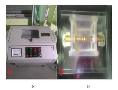
Fig. 4. 100kV BDV test Kit and Oil test cell
