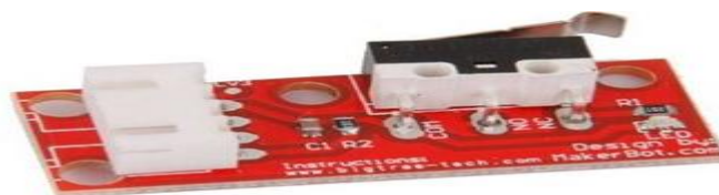
Figure 5: End Stop Switch
